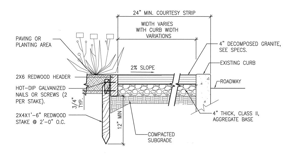
DECOMPOSED GRANITE PAVING OPTION IN COURTESY STRIP SCALE: 1"=1'-0"
