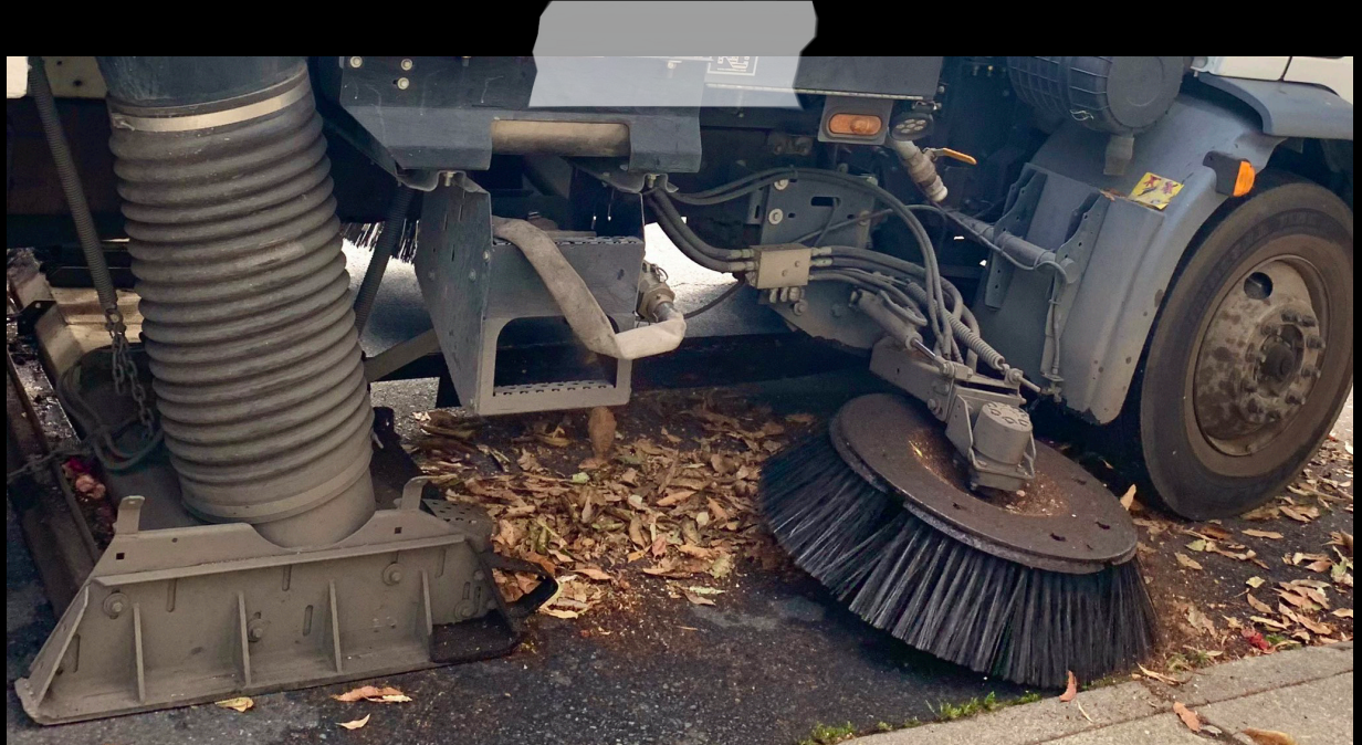
OUR MECHANICAL SWEEPER REMOVES LEAVES AND LITTER FROM A SAN FRANCISCO STREET.
